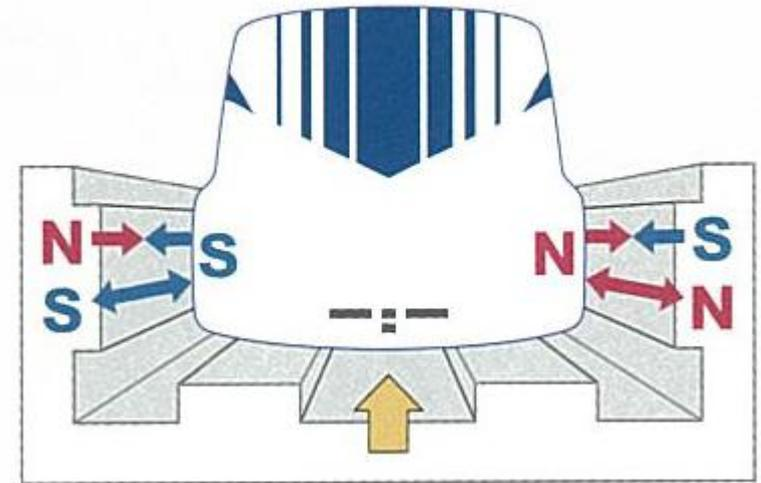
Levitation and Guidance forces are produced by interaction (repulsive or propulsive) between Guideway Track on the ground and Superconducting Magnets built in the vehicle when it passes through at high speed..
