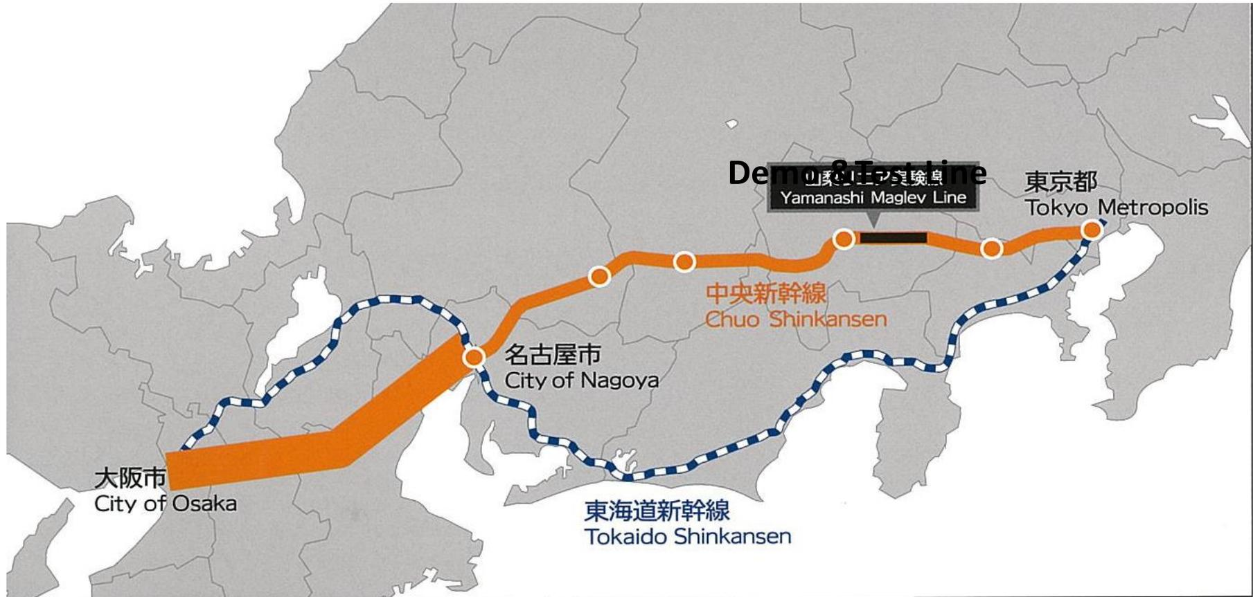
Target: 500 km/h to run Tokyo/Osaka in 67 min.
