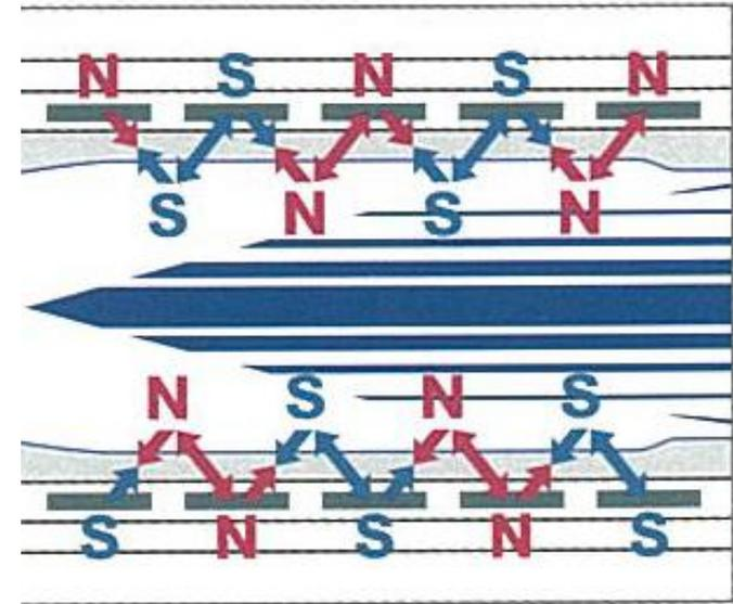
Propulsion force is produced by interaction (repulsive or propulsive) between Propulsion Coils on the ground and Superconducting Magnets built in the vehicle.
