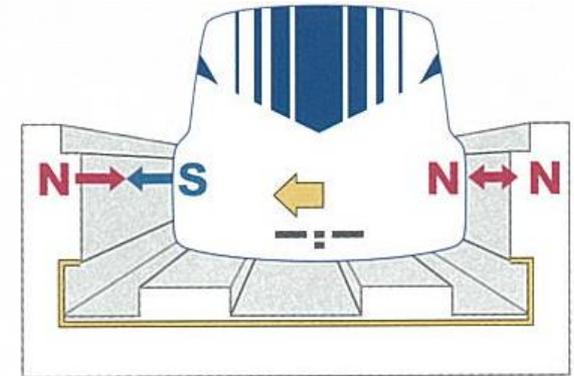
Levitation & Guidance Coils on the guideway keep the vehicle by attractive force (far side) and repulsive force (near side) to keep the vehicle in the center of the guideway.
