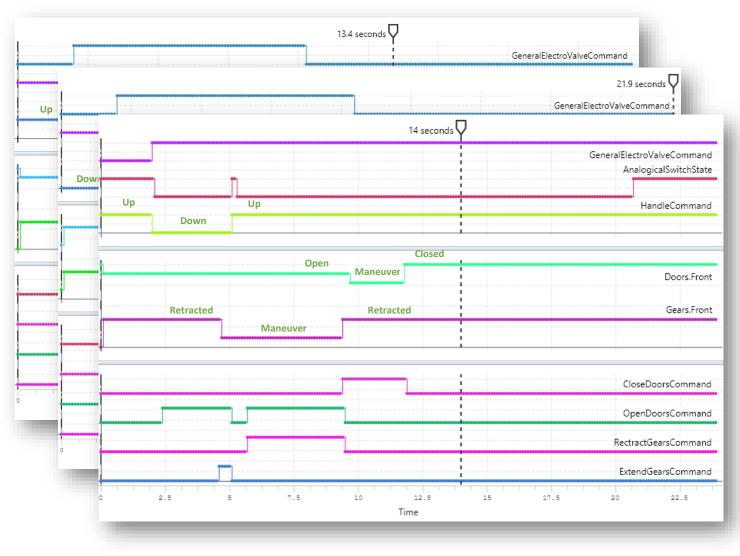
When handle becomes down, gears go from the retracted to extended position, and doors from (already) open to closed
