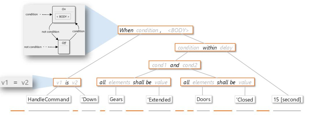
When HandleCommand is 'Down, all Gears shall be 'Extended and all Doors shall be 'Closed within 15 [second]
