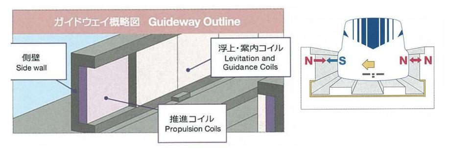
Levitation & Guidance Coils on the guideway keep the vehicle by attractive force (far side) and repulsive force (near side) to keep the vehicle in the center of the guideway.
