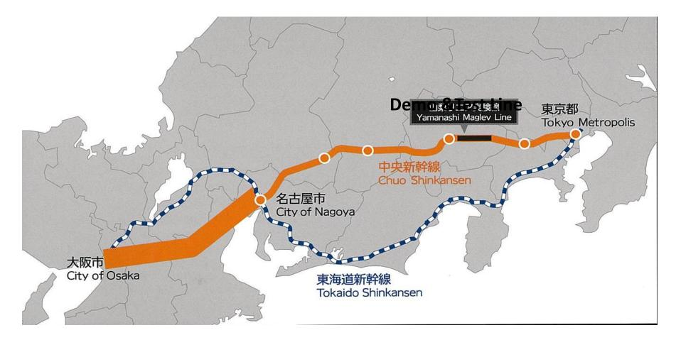
Target: 500 km/h to run Tokyo/Osaka in 67 min. And Provision against E/Q, Tsunami & Eruption
