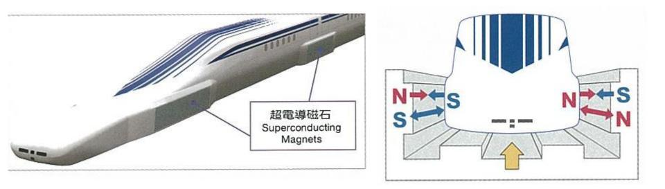
Levitation and Guidance forces are produced by interaction (repulsive or propulsive) between Guideway Track on the ground and Superconducting Magnets built in the vehicle when it passes through at high speed..
